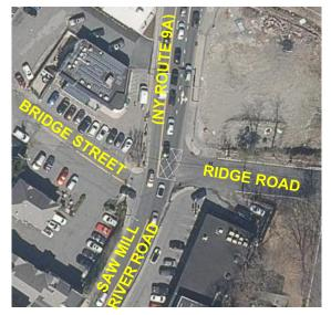
The intersection of Ridge Road and Site Driveway C is a three-legged unsignalized intersection. Ridge Road provides a single lane for both the eastbound and westbound approaches for thru and turning movements. Site Driveway C is the existing driveway along Ridge Road which provides a single lane for left and right turns. Under proposed conditions, this driveway would removed.
