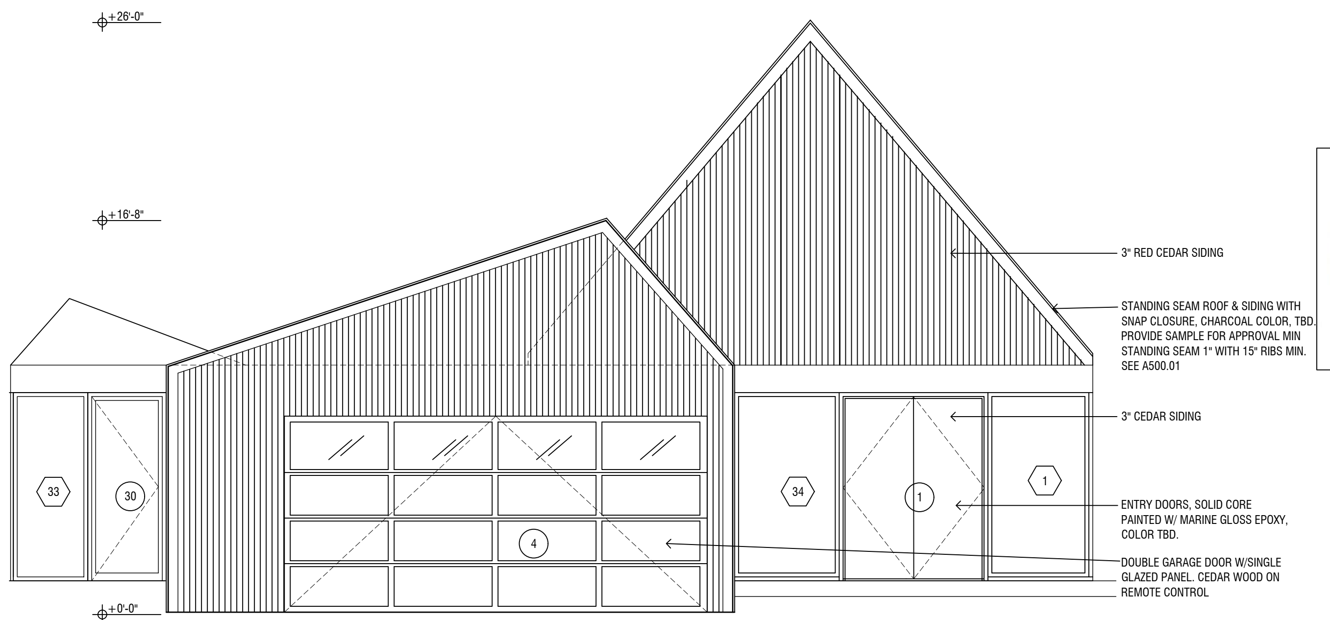
1 ELEVATION - FACING NORTH EAST
