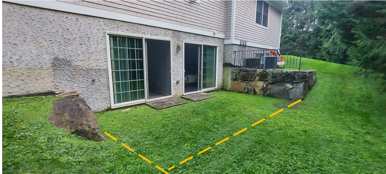
Rear Yard/ Basement Doors: Dashed lines indicate extents of proposed wood decking at door sill level
