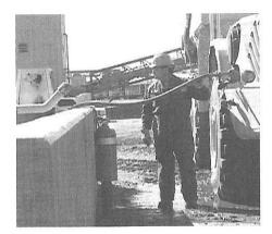
S tay with your vehicle while fueling to avoid overfilling or the hose falling out of the filler pipe.
