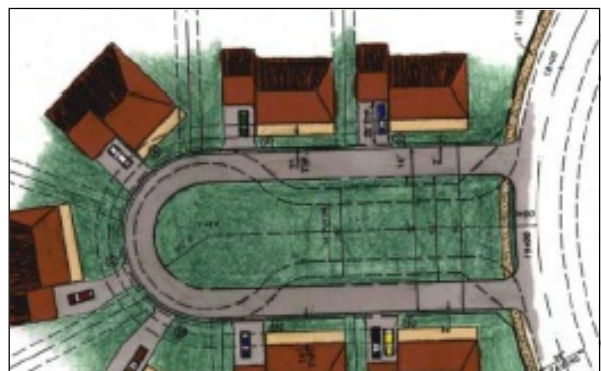
Figure 5.23 Loop road option (Source: Center for Watershed Protection, 2005)
